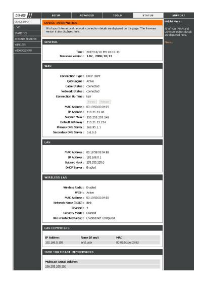
Note: Because a dynamic WAN IP can change from time to time depending on your ISP, you may want to obtain a Static IP address from your ISP. A Static IP address is a fixed IP address that will not change over time and will be more convenient for you to use to access your camera from a remote location. The Static IP Address will also allow you to access your camera attached to your router over the Internet.
